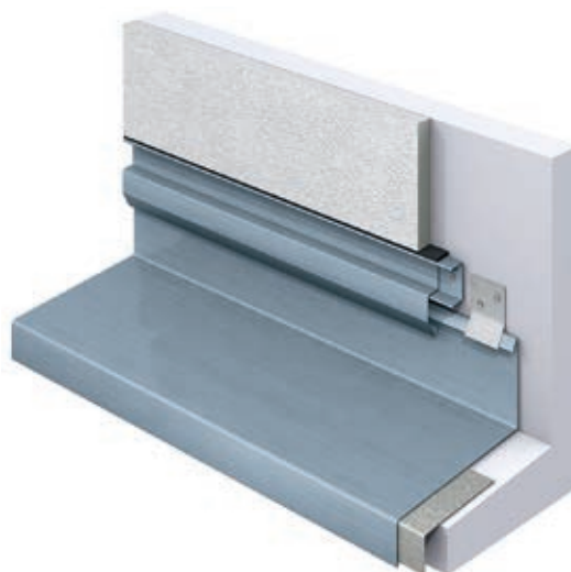
Fig. 25: Render flashing with cover flashing
