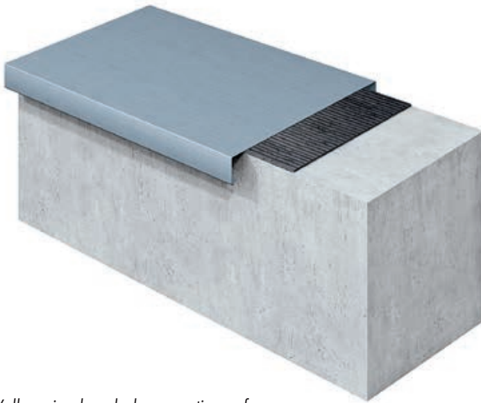
Fig. 5: Wall coping bonded over entire surface
