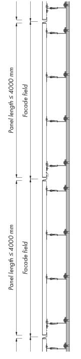
Example A: Facade field joint (separation by means of expansion joints)
