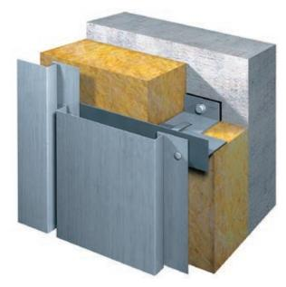
Double or two-part substructure
